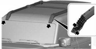
4. Position the roof rack on the vehicle.
